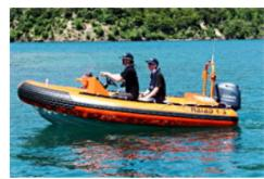
The Naiad twin pontoon system of butyl rubber inners covered by extra heavy duty PU/PVC outers are easily removable and replaceable anywhere in the world. Naiad has concentrated on "in the field" maintenance because Naiads are used in such out of the way places, from the South Pacific to Antarctica and Alaska
