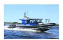
Two of these craft are being used in Australia by the Queensland Police as Patrol boats in the Gladstone and Brisbane areas. These boats use Naiad's popular 11.3m stepped hull, with a large enclosed crew cabin. The same Naiad stepped hull technology is also used in the 9m and 10m Coastguard boats and many of the 12.5m tourist boats.
