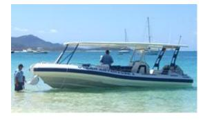
Powered by twin 150 h.p. outboards, the craft's top speeds are 41 knots (lightly laden) and 35 knots (with full load). With comfortable, economical cruising around 25-30 knots, this is the ideal craft for long distance, nine metres being the ideal boat length for traversing choppy seas generated by high winds.
