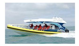
Deck layout is customised to the needs of the tour operator, but the general arrangement has the majority of passengers up front and the drivers station, which is raised, at the rear. The RHIB design means the pontoons are low to the deck and coupled with tiered cinema style seating offers an excellent view for the passengers from every seat.
